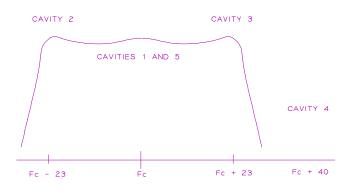
Figure 1 Frequencies of cavities, C-band klystrons. C:\BrianS\MARKETIN\Klystron\Publications\KLYTUNE.doc
