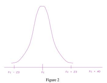
Synchronously tuned gain response.
